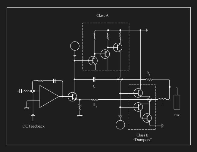
"Bridge": L, C, R &  $R_2$ Bridge is balanced when  $L = R_1, R_2, C$
